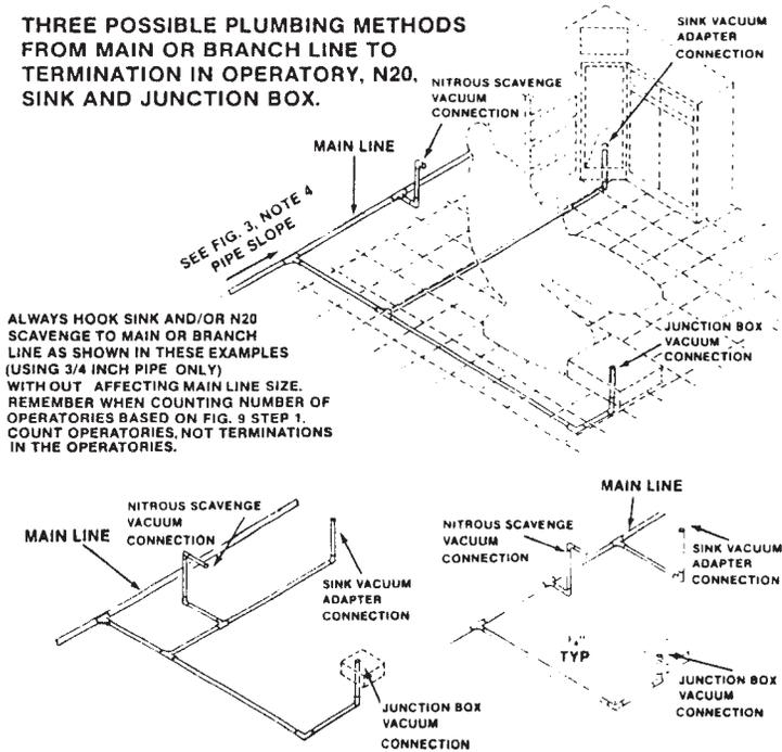
ALWAYS HOOK SINK AND/OR N20 SCAVENGE TO MAIN OR BRANCH LINE AS SHOWN IN THESE EXAMPLES (USING 3/4 INCH PIPE ONLY) WITHOUT AFFECTING MAIN LINE SIZE. REMEMBER WHEN COUNTING NUMBER OF OPERATORIES BASED ON FIG. 9 STEP 1. COUNT OPERATORIES, NOT TERMINATIONS IN THE OPERATORIES.
